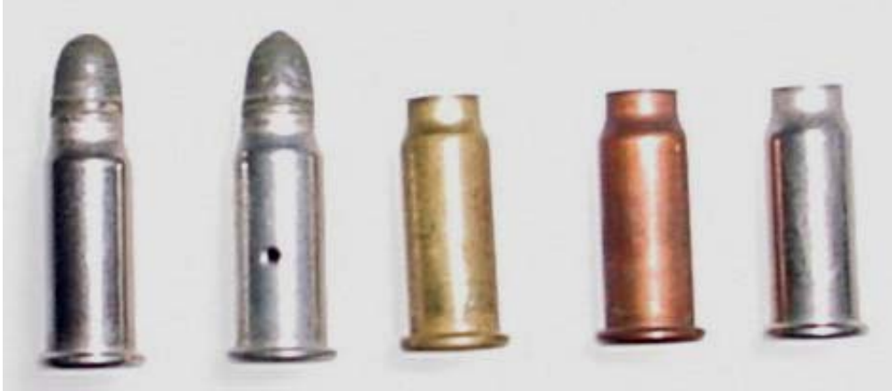
Fig. 4: .17 High Standard Rimfire cartridges that came with the gun. Left to right: ball, dummy, brass case, copper case & nickel case
