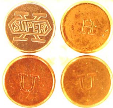
Fig. 5: .17 High Standard Rimfire headstamps that came with the gun. Left to right: Super X on nickel case, H on brass case, and bottom are U headstamps on both copper and brass cases
