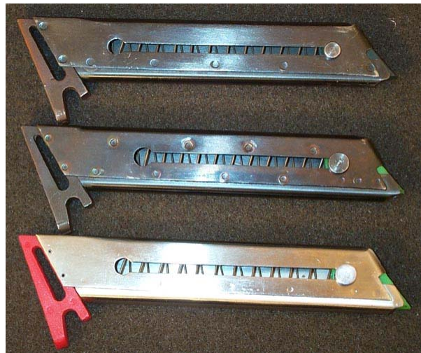
Figure 6 right side view of magazines From top to bottom: Old Triple K, New Triple K, Mitchell
